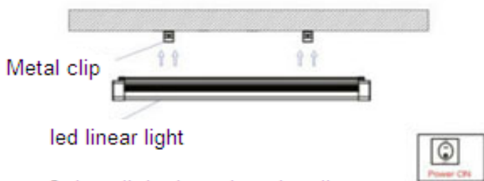
C. Install the lamp into the clips
